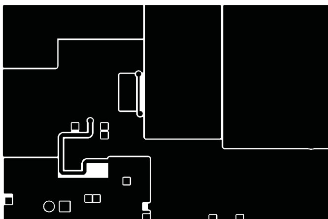
Figure 46. TPS40200EVM-001 Bottom Copper (X-Ray View from Top)
